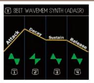
This is the ADSAR mode of the 8-bit waveform memory synth. The waveform changes according to the envelope position.
