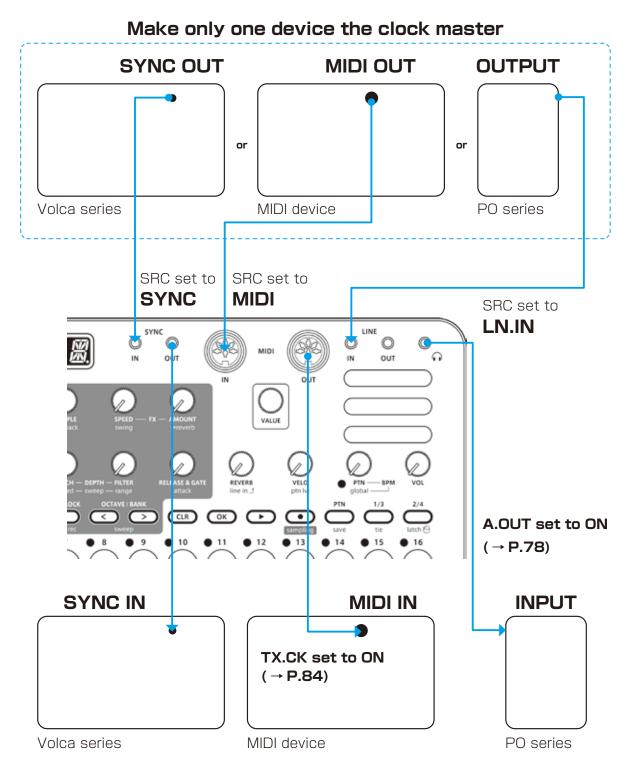
Using the bridging function, it is possible to synchronize devices with different connectors. For example, a Pocket Operator acting as a clock master can be used to synchronize a Volca or MIDI device connected to the Lofi-12.
