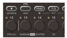
In the example above, the secondary functions of the  $\stackrel{\text{\tiny TD}}{\hookrightarrow}$  and  $\stackrel{\text{\tiny L}}{\circlearrowleft}$  buttons are "save" and "RANDOM".
