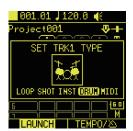
Turn be to select a preset pattern. By pressing be while turning it, preset patterns can be switched by genre. For this example, select the **ROCK 01** pattern.
