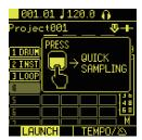
Make an effect sound, such as a hand clap. Recording will start automatically if the level exceeds the AUTO REC level setting.
