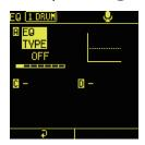
Use ⊕ A to select the EQ type and use ⊕ c and ⊕ P to adjust the parameters.
