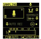
2 Turn the mic gain knob to adjust the gain. Adjust it so that the level meter exceeds -12 dB when the effect sound, such as a hand clap, is made.
